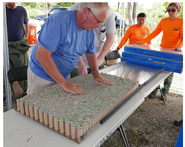
Fig. 3 Bait cartridges are inspected for manufacturing imperfections or shipping damage that might impede smooth feeding and ejection.
