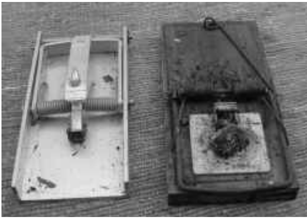
Fig. 1 Relative condition of Ka Mate prototype (left) and Victor Professional (right) after equal environmental exposure at adjacent sites in the Big Bush trap trial.
