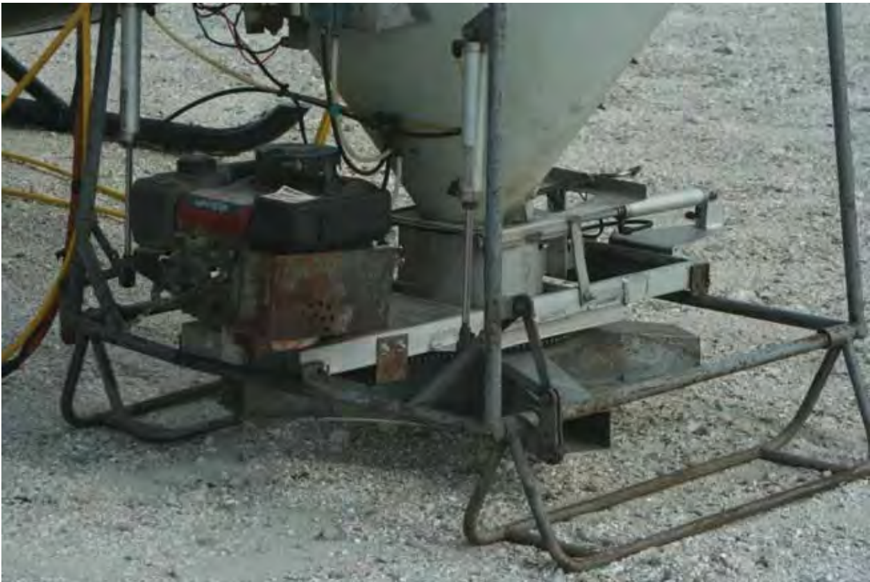
Figure 7. The bait spreader mechanism, with drive motor on the left.
